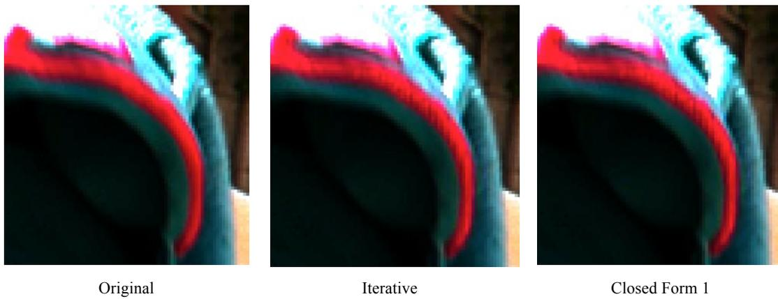
Figure 8. Sequence Market. Mismatch between chroma upsampling filters. Comparison of Iterative algorithm and Closed Form 1 solution with the original.
