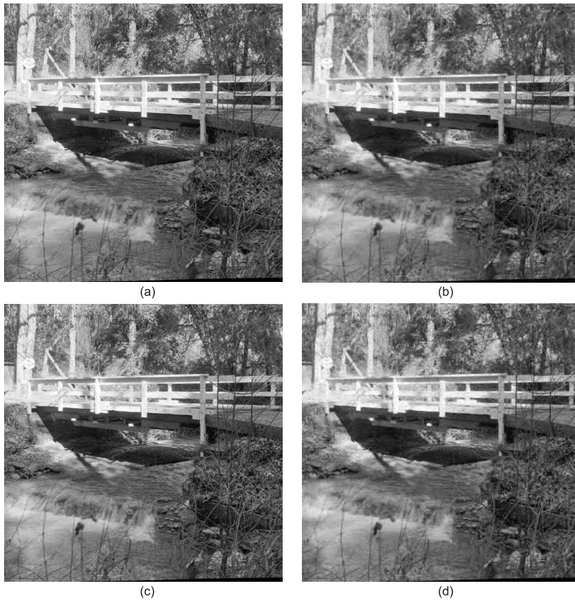
Fig. 19. Reconstructed image “Stream and bridge”, spline interpolation and DCT coding of shaper. DCT coding of the residual ( R = 1.700 bpp, \rho = 14.7\% ): (a) reconstruction from both descriptions, D_0 = 32.10 dB; (b) reconstruction from Description 1, D_1 = 26.52 dB. LOT coding of the residual ( R = 1.705 bpp, \rho = 14.7\% ): (c) reconstruction from both descriptions, D_0 = 31.58 dB; (d) reconstruction from Description 1, D_1 = 25.63 dB.
